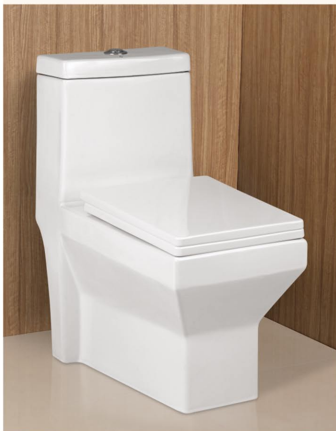
▼ No.6184 Siphonic one piece toilet Size : 755 x 685 x 370mm S trap 300mm Roughing - in Outer Diameter 100mm
