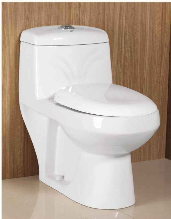
▼ No.2065 wash down one piece toilet Size : 690 x 650 x 375mm S trap 100,200mm Roughing - in Outer Diameter 100mm
